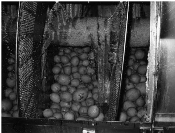
FIGURE 4.5 (See color insert following page 468.) “Pellatrici method.” The spiked Archimedes screw with lemons, washed with water.
