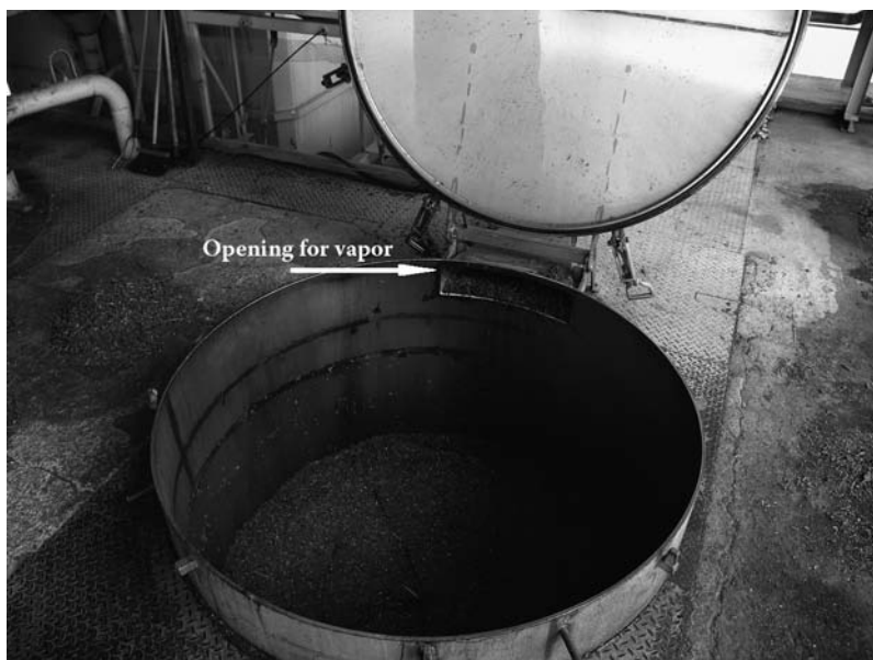
FIGURE 4.12 Open kettle with opening for vapor and oil.
