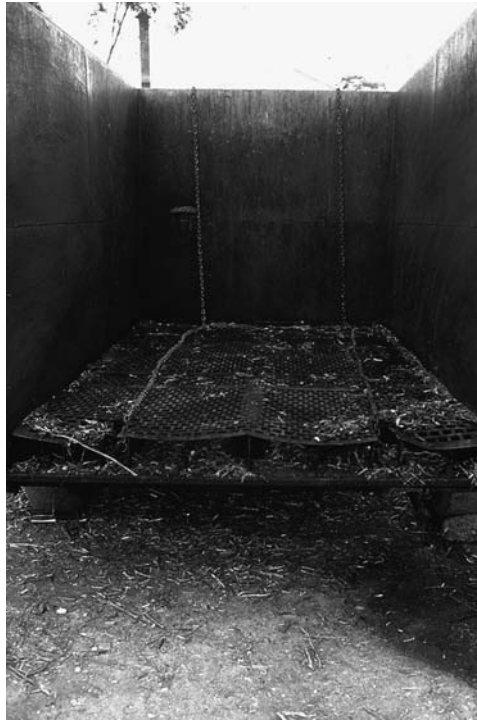
FIGURE 4.23 View inside the distillation container, showing the steam tubes and the metallic grid.
