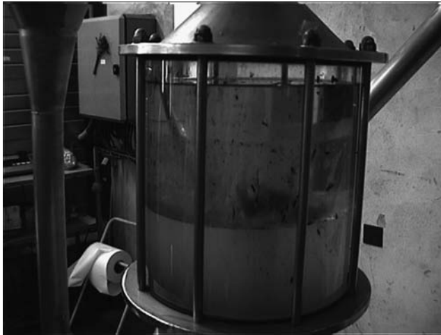
FIGURE 4.18 (See color insert following page 468.) Oil and muddy water in the Florentine flask.
