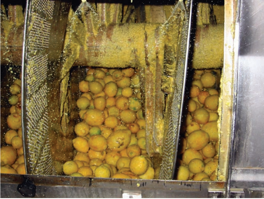
FIGURE 4.5 “Pellatrici method.” The spiked Archimedes screw with lemons, washed with water.
